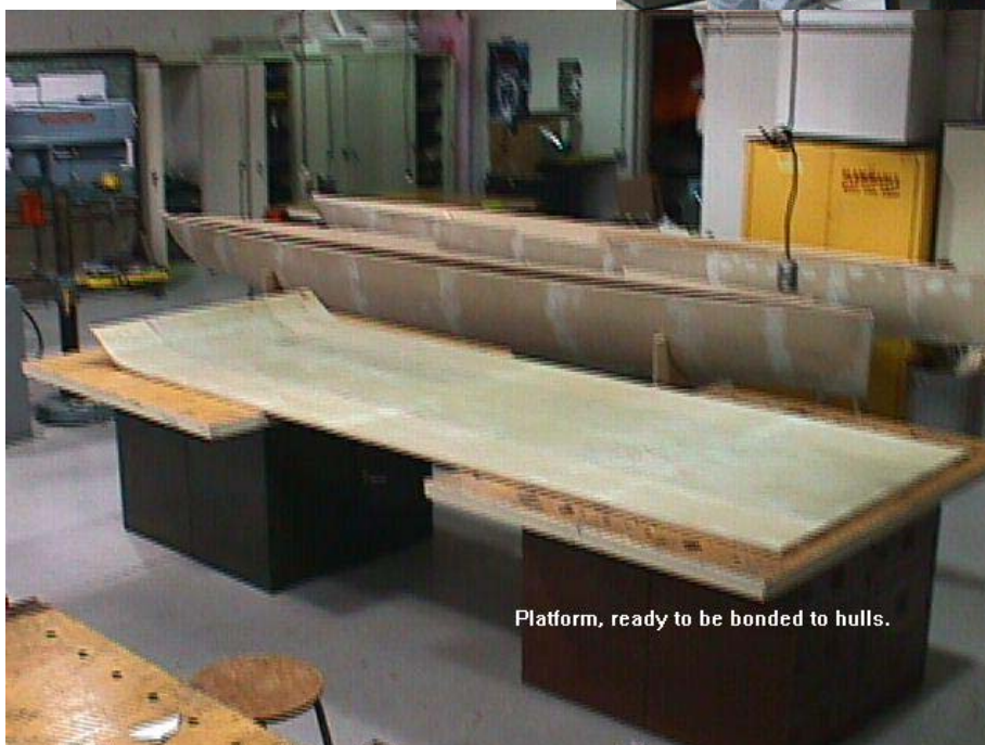
James preping plug to lay-up the platform which will connect the two hulls of the catamaran.
