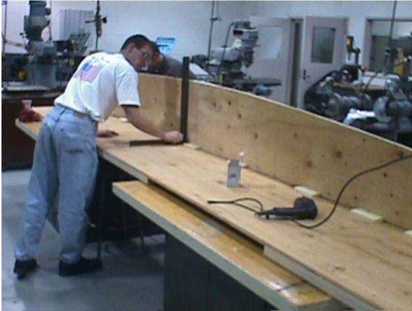
James setting the keelson for the hull plug.
